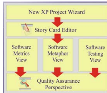
Fig. 1. Block Diagram for ADEPT: Shows all the plug-ins that constitutes that project management tool along with their dependencies representing the complete SDLC cycle
