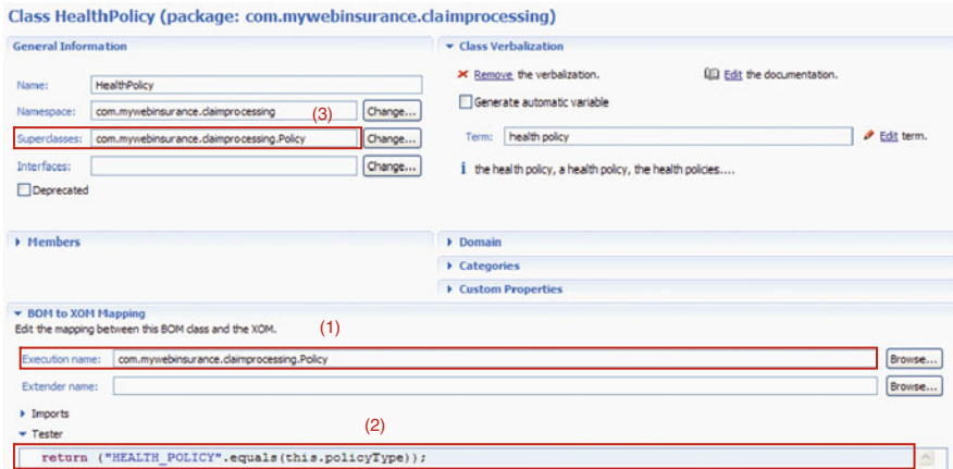
Fig. 10.15 BOM editor for BOM classes. To define a virtual BOM class, we need to (1) specify its execution name (i.e., corresponding XOM class), (2) specify what conditions instances of the XOM class need to satisfy (tester), and (3) specify its BOM superclasses
