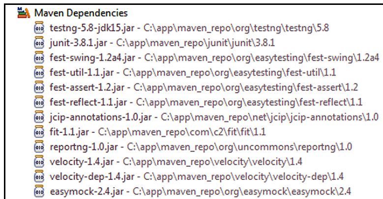
Figure 6.2 M2eclipse manages the Eclipse Maven classpath container. In your Eclipse project, all JARs are referenced as binary dependencies. No manual referencing or checking of artifacts is needed, and the approach is congruent, both in your workspace (IDE) and in your build script.
