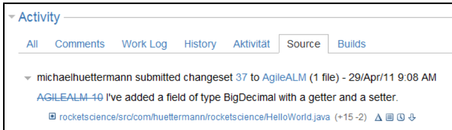
Figure 4.8 FishEye integrated into JIRA: A dedicated tab shows source changes associated with each ticket. One Subversion commit resulted in this entry: 1 file was changed, 15 lines were added in the file, and 2 were removed. Icons provide links to FishEye so you can zoom in if you're interested in more information.
