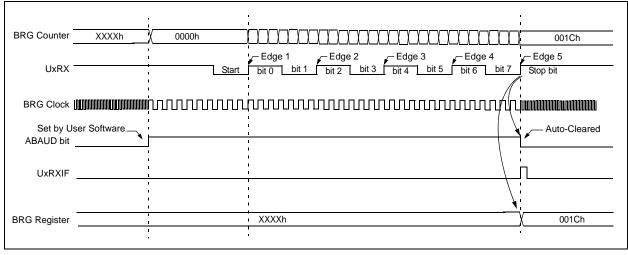
While the auto-baud sequence is in progress, the UART state machine is held in the Idle state. The UxRXIF interrupt is set on the 5th UxRX rising edge, independent of the URXISEL<1:0> settings. The receiver FIFO is not updated. 17
