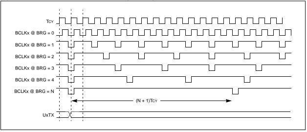
Figure 17-2: BCLKx Output vs. UxBRG Programming
