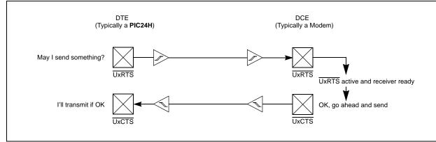
Figure 17-18: UxRTS/UxCTS Bus Enable for IEEE-485 Systems (RTSMD = 1)
