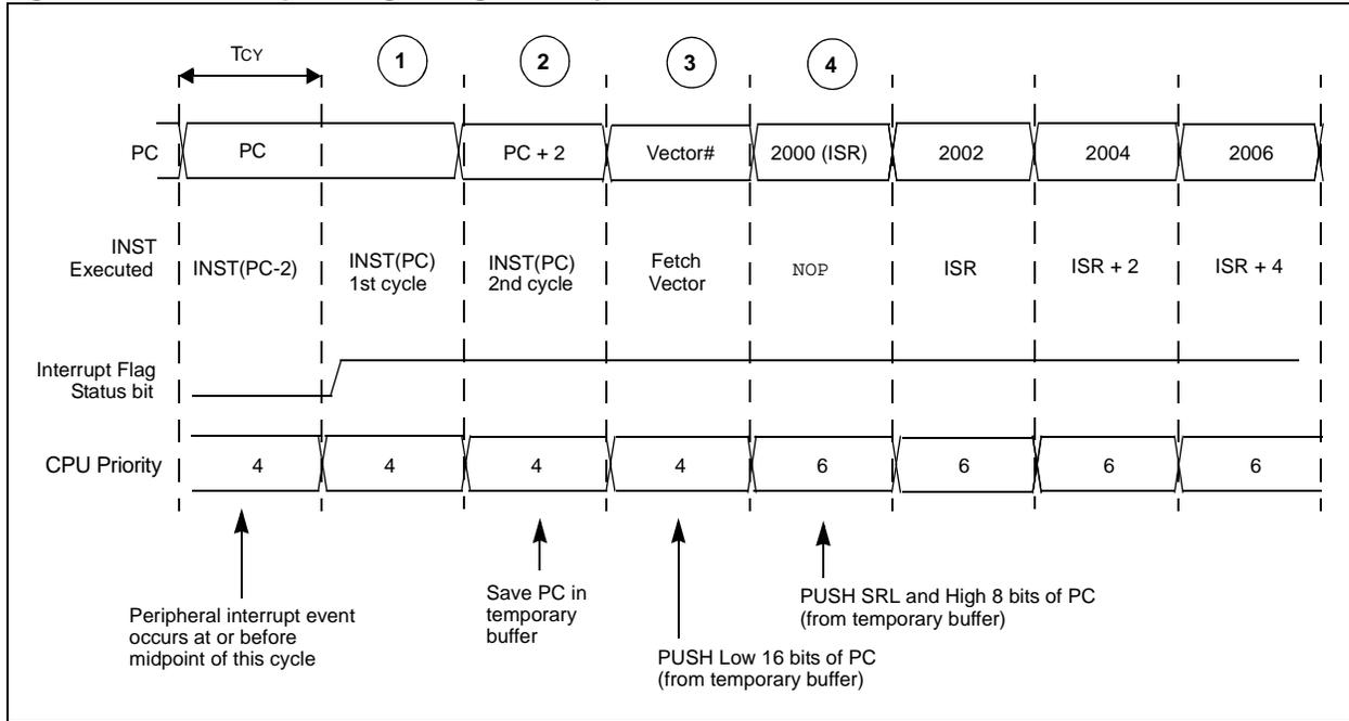
**Figure 6-5: Interrupt Timing, Interrupt Occurs During 1st Cycle of a Two-Cycle Instruction**
