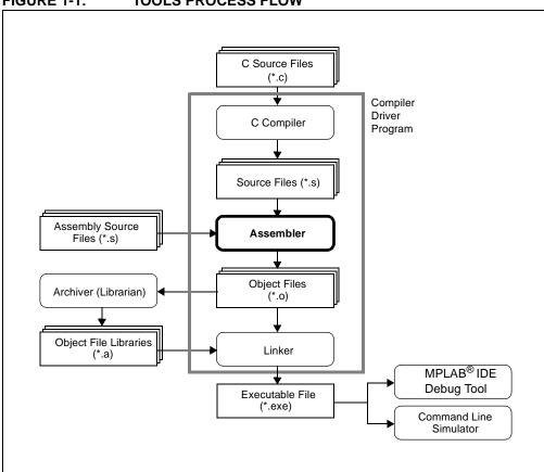
FIGURE 1-1: TOOLS PROCESS FLOW
