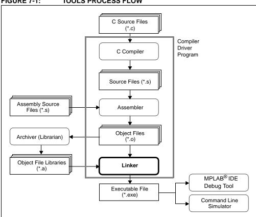
FIGURE 7-1: TOOLS PROCESS FLOW
