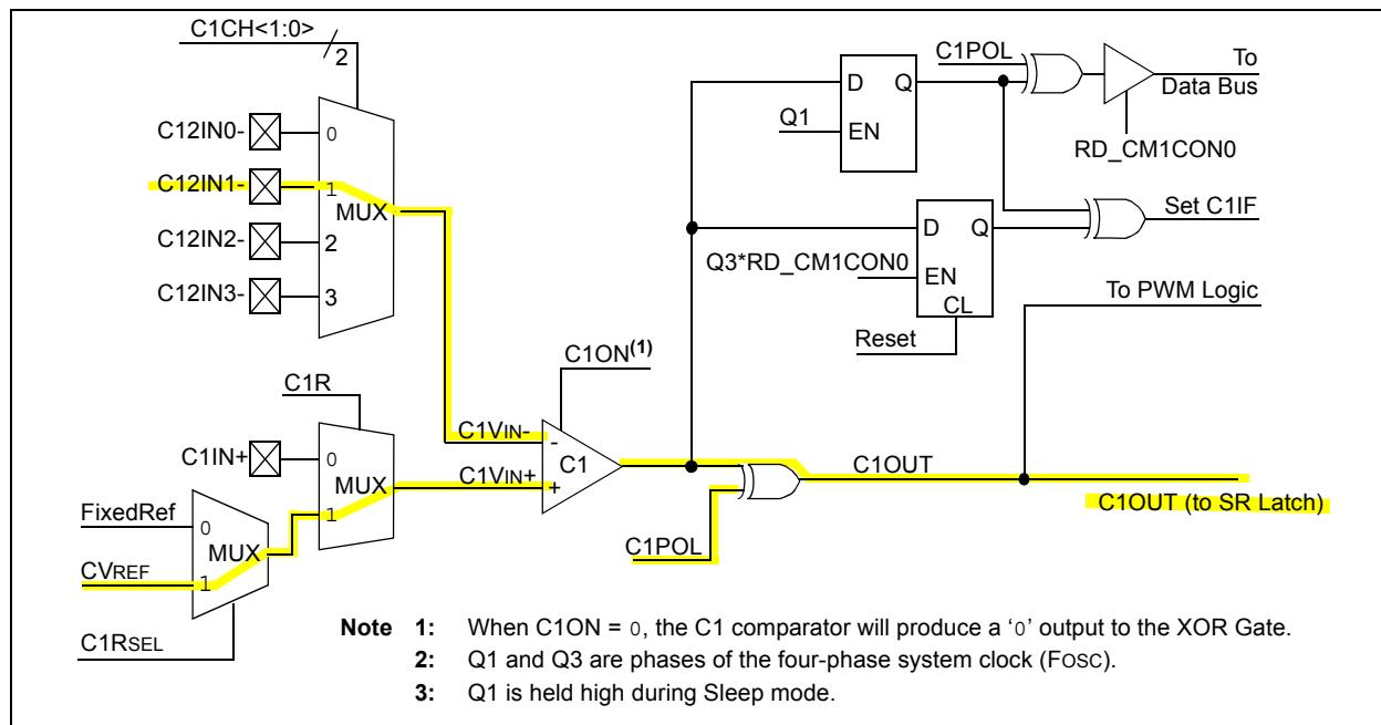
\* Comparator modules capable of touch sense as described must have the SR-latch option.
