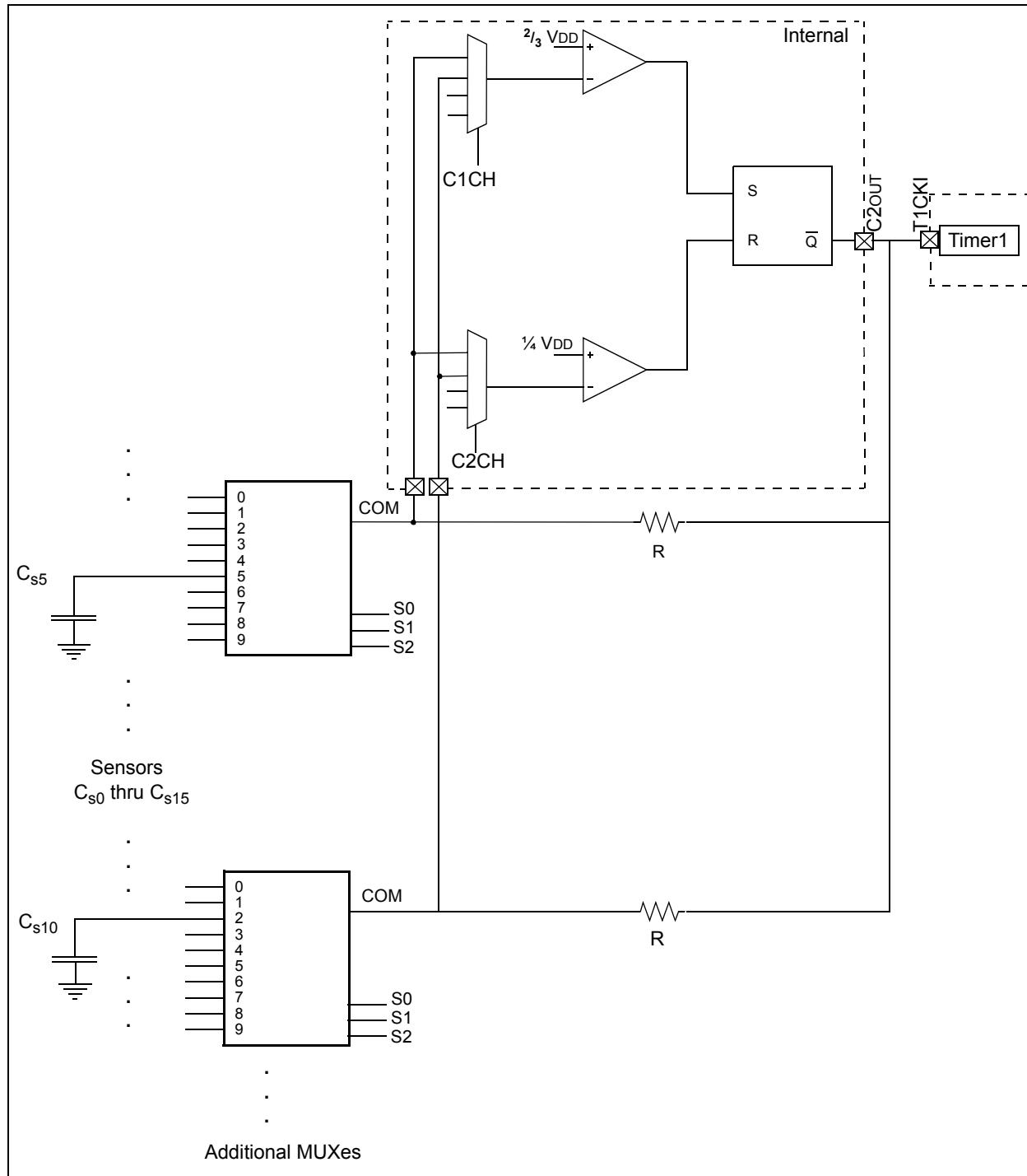
In addition to enabling the external MUX and its control lines, the appropriate comparator input must be selected for the internal 4-channel MUX. Because of the definition of MUXx on C12INx- chosen before, the integer division index/8, conveniently also yields the comparator input channel bits to select for C1CH and C2CH. The following code example shows how to scan 32 buttons as in the described configuration.
