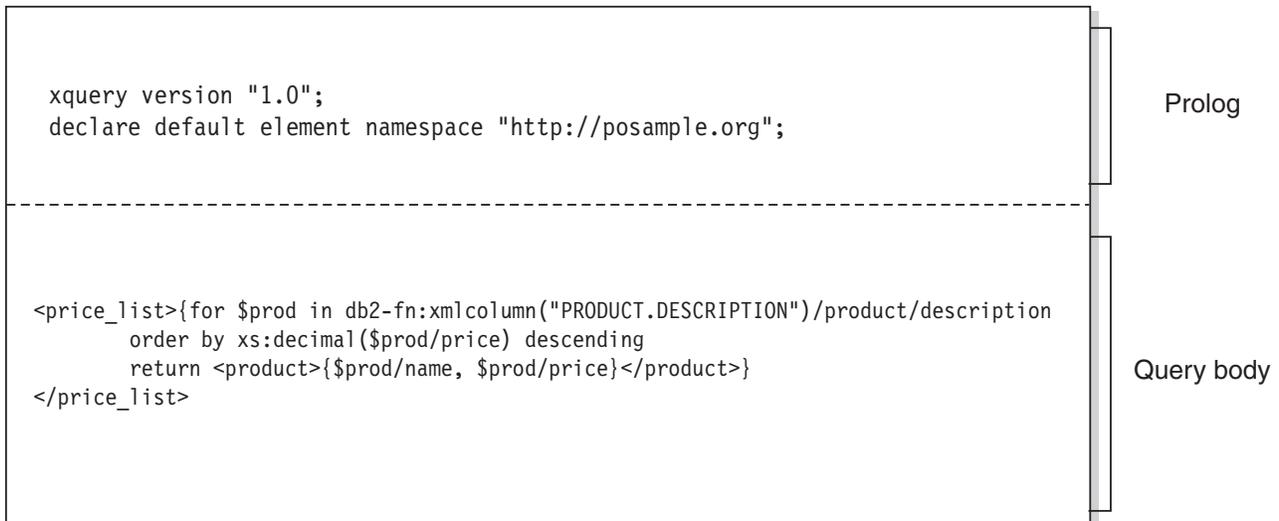
Figure 1. Structure of a typical query in XQuery
